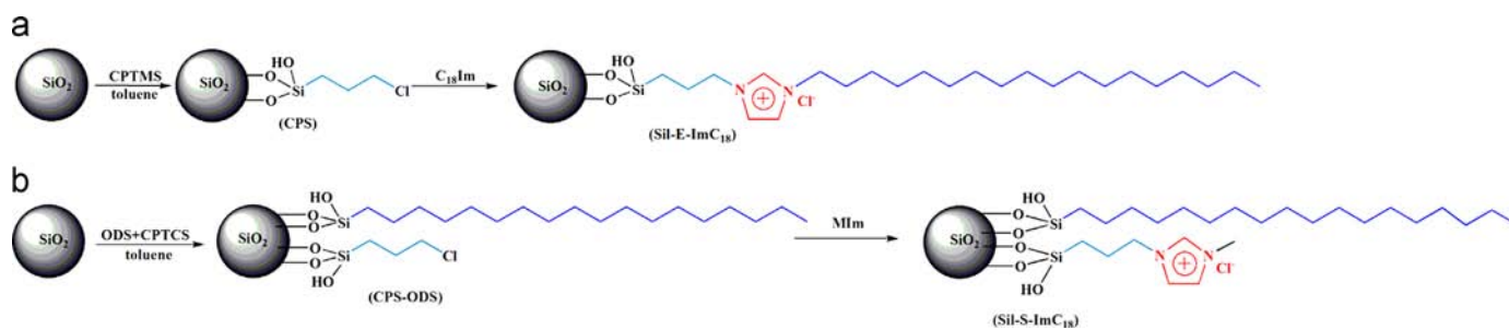
Fig. 1. Synthetic strategy for imidazolium-functionalized polar-embedded (a) and polar-spaced (b) stationary phases.
